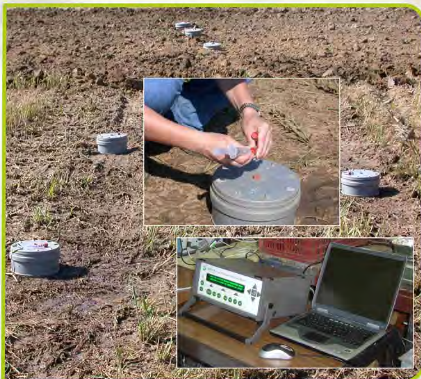
Figure 15 - Measurement of gas fluxes ( \text{CO}_2 , \text{CH}_4 e \text{N}_2\text{O} ) from soils amended with organic residues.
