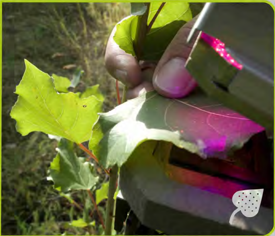
Figure 9 - Measurement of CO 2 assimilation by plants in the field.
