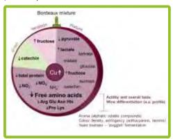
Effect of Bordeaux mixture application in grape berry metabolic composition (arrows indicate variations in solute levels), and parameters affected by excess copper in must and wine.
