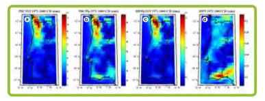
Extreme Precipitation indices for Continental Portugal. Values of the (a) long-term 95<sup>th</sup> percentile (PRC95p), (b) total precipitation (PRCTOT), (c) total precipitation falling in days with daily precipitation amounts greater than the corresponding PRC95p (RR95pTOT) and (d) the ratio between RR95pTOT and PRCPTOT (R95T) evaluated for daily precipitation simulated by the COSMO-CLM model, for recent–past climate conditions (C20 scenario, 1971 – 2000).
