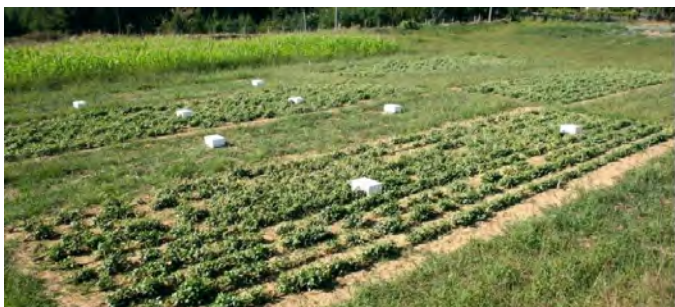
Field trials in UTAD with chambers for sampling gas emissions from soil in the Summer (cowpea crop and fallow plots ; on the left) and in the Winter (triticale crop; on the right).
