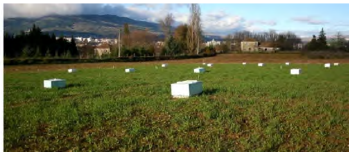
Field trials in UTAD with chambers for sampling gas emissions from soil in the Summer (cowpea crop and fallow plots ; on the left) and in the Winter (triticale crop; on the right).
