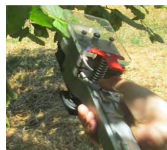
Leaf gas exchange asurements with IRGA
