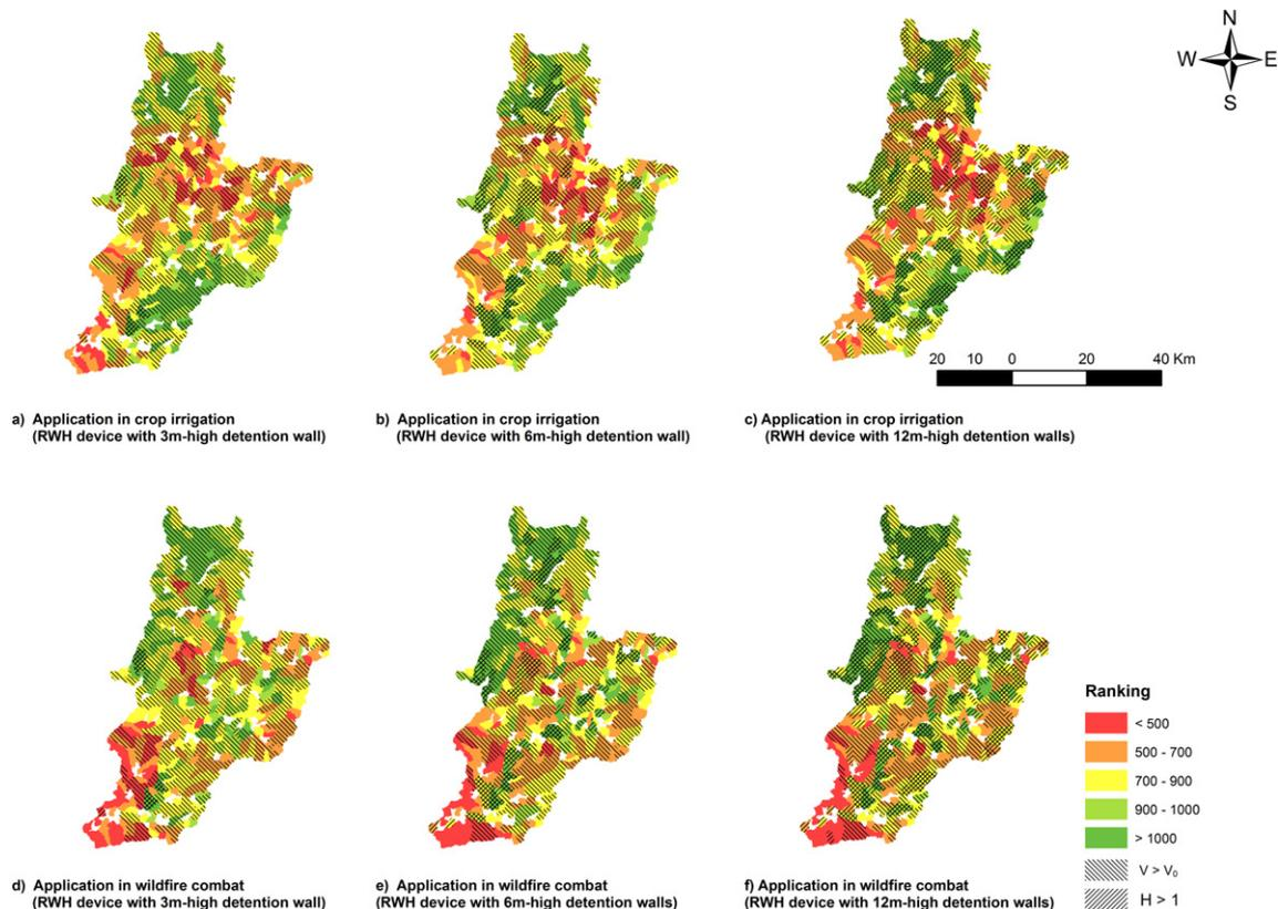
Fig. 7. Results of ranking analysis, considering the building of 3, 6 and 12 meter high dam walls and the application of harvested rainwater in irrigation and wildfire combat.
