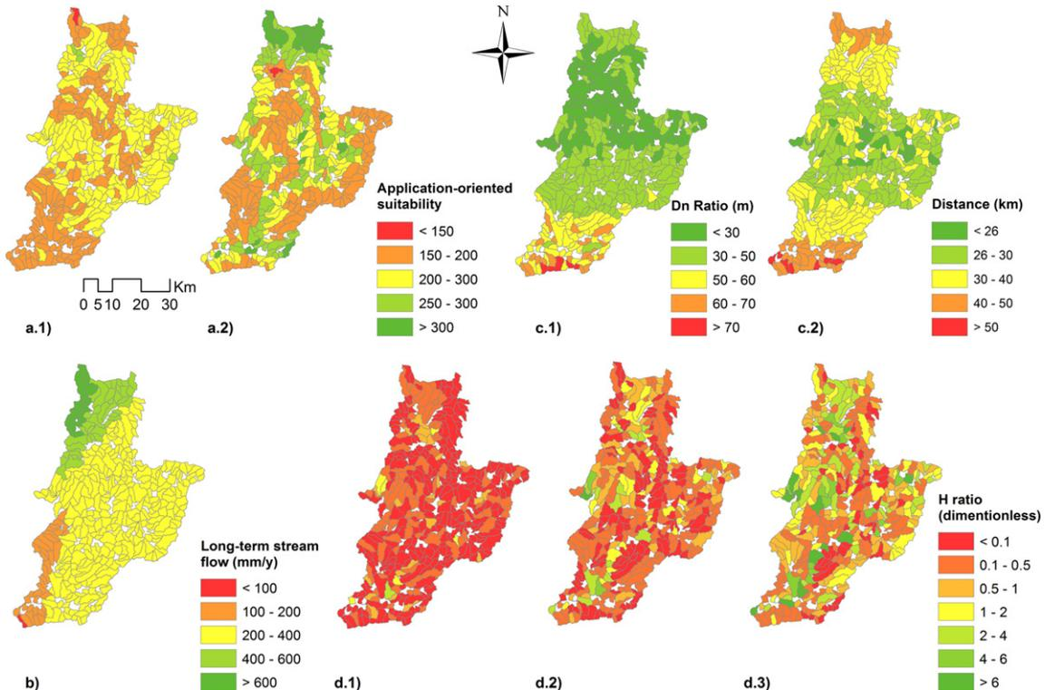
**Fig. 6.** Spatial distribution of application-oriented suitability (6a), long-term stream flow (6b), and allocation parameters (6c, 6d), averaged within 384 sub-catchments.
