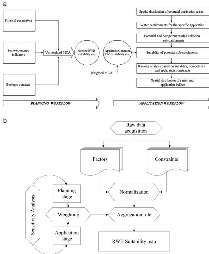
**Fig. 2.** a – Rainwater harvesting (RWH) suitability model, comprising the planning and allocation workflows. The details on the model are provided in the text. Adapted from Terêncio et al. (2017). b – Flowchart describing the spatial Multi Criteria algorithm embedded in the RWH suitability model (Fig. 2a). Adapted from Terêncio et al. (2017).
