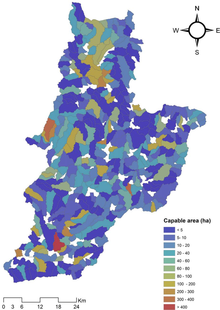
Fig. 8. a – Spatial distribution of irrigable areas supplied by a 3 meter high dam reservoir. b – Histogram of irrigable areas supplied by a 3 meter high dam reservoir.
